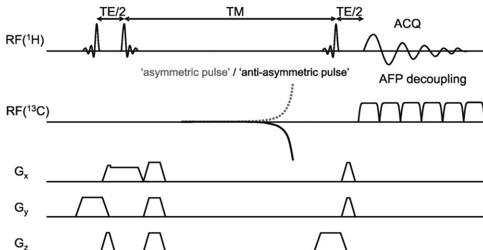
FIG. 1. Selective resonance suppression  $^1\text{H}$ - $^{13}\text{C}$  NMR sequence (RACED-STEAM). Two asymmetric adiabatic inversion pulses are applied in the  $^{13}\text{C}$  channel on alternate scans, where the direction of the adiabatic sweep is alternated (indicated by the dashed line). Broadband adiabatic decoupling is applied during the acquisition.
