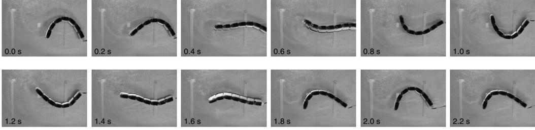
Fig. 2. The robot swimming in water with the optimal parameters ( $A = 40^\circ$ ,  $N \cdot \Delta\phi = 0.25$  and  $\nu = 0.5$  Hz).
