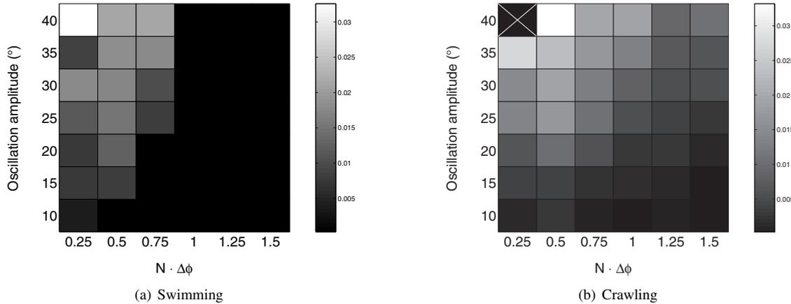
Fig. 4. Locomotion characterization at  $\nu = 0.25$  Hz. The cross in the second plot corresponds to parameters that cause the robot to fall over.
