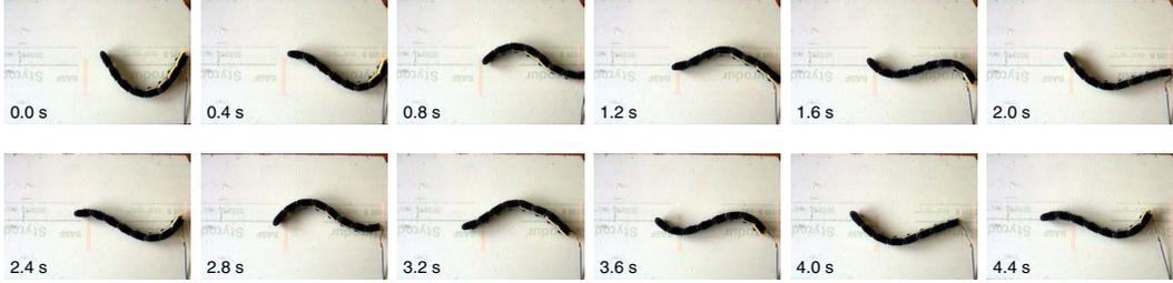
Fig. 3. The robot crawling on ground ( $A = 30^\circ$ ,  $N \cdot \Delta\phi = 0.5$  and  $\nu = 0.5$  Hz).<sup>1</sup>
