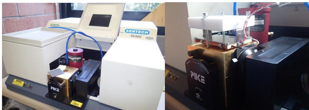
Figure 1: Bio-Rad FTS-175C FTIR spectrometer equipped with the golden integrating sphere, MCT detector for the Mid-IR range and the designed heating stage.
