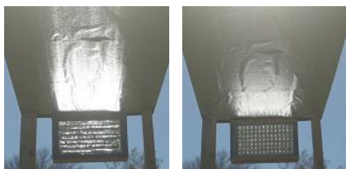
Figure 10: Peak Brightness of Prototype Under Direct Sun Without Rods (Left) and With Rods (Right)
