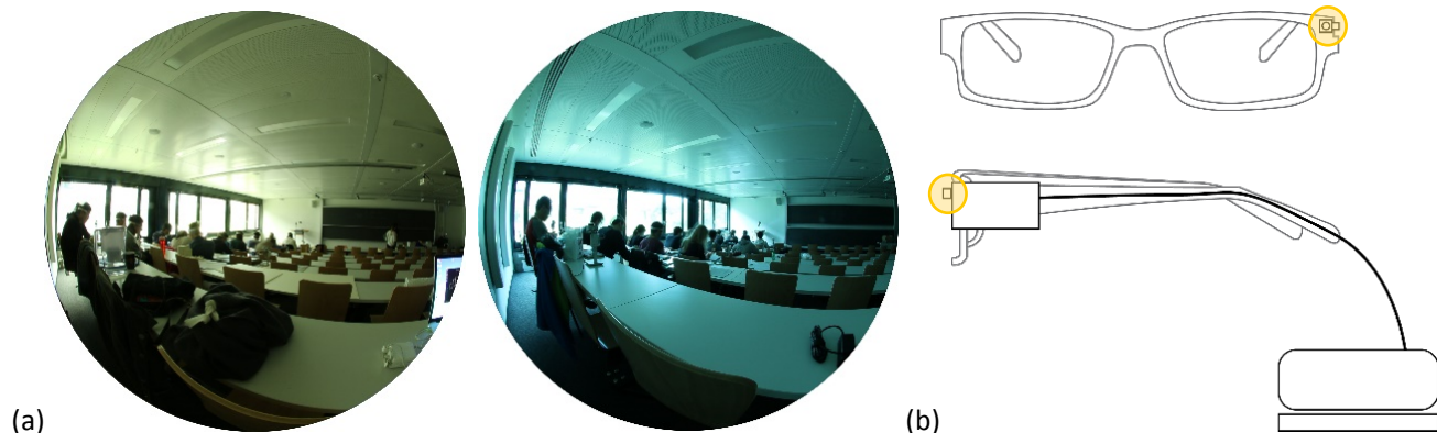
Figure 1. (a) Experimental design. Control group experienced daylight neutral conditions (left) and intervention group experienced redimpoveryed daylight (right). (b) SMEAS, customized wearable device to measure vertical illuminance and irradiance.
