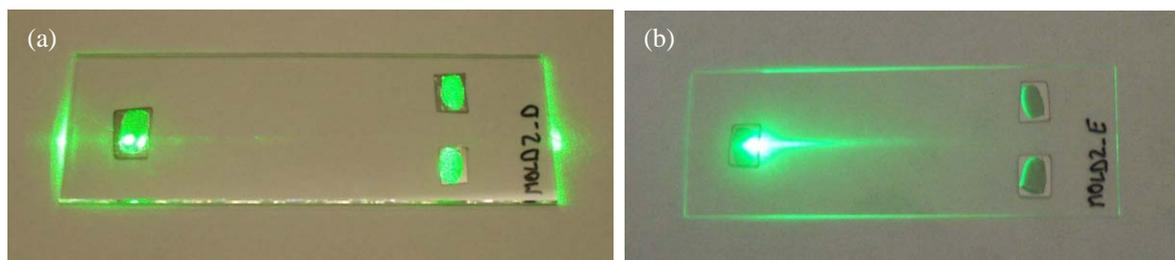
Fig. 4: Optical picture of 25 x 70 mm (a) glass and (b) 100  $\mu\text{m}$  thick PET waveguides. Light from a laser was applied to the left mirror and came out of the measurement and reference channels on the right, which showed the proper optical operation of the device.
