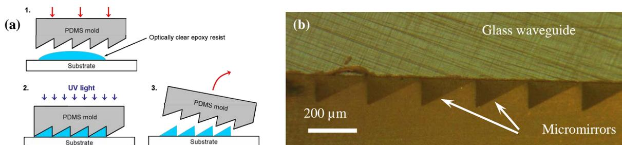
Fig. 2: (a) Patterning of a UV-curable resist. A droplet of resist was dispensed on the substrate (1) before molding it with a PDMS part (2). The resist was polymerized by UV light before removing the mold (3). (b) Cross-sectional picture of the micro-mirrors patterned on glass slide.
