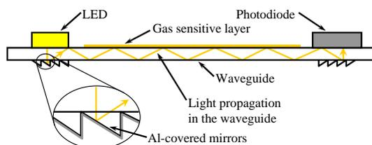
Fig. 1: Cross-sectional schematic of the transducer. A LED was used as light source. The light intensity that reaches the photodiode (i.e. the sensor response) depends on the absorption of light in the evanescent field going along the colorimetric film in presence of the gas to be detected.
