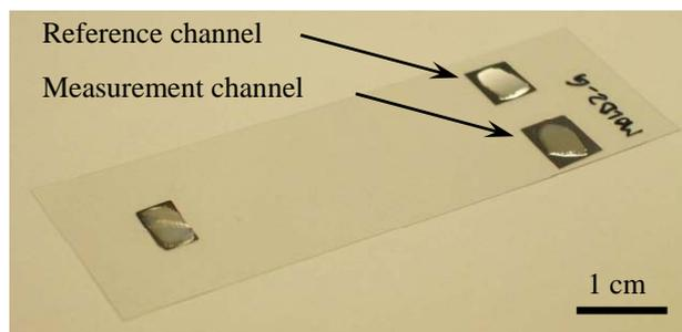
Fig. 3: Optical picture of a PET optical waveguide with micro-mirrors covered with 300 nm of aluminum.
