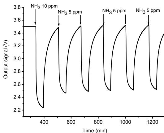
Fig. 5: Gas measurement performed with the colorimetric sensor consisting in a 250  $\mu\text{m}$  thick PET foil with uncovered mirrors when exposed to different concentrations of  $\text{NH}_3$ . The measurement was carried out in synthetic air with about 50% of relative humidity and a gas flow of 500 ml/min.
