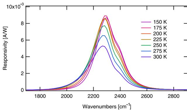
**Fig. 3** Responsivity curves of a 4.4 μm QCD as a function of temperature. The little bump around 2330 cm<sup>-1</sup> is due to CO<sub>2</sub> absorption bands
