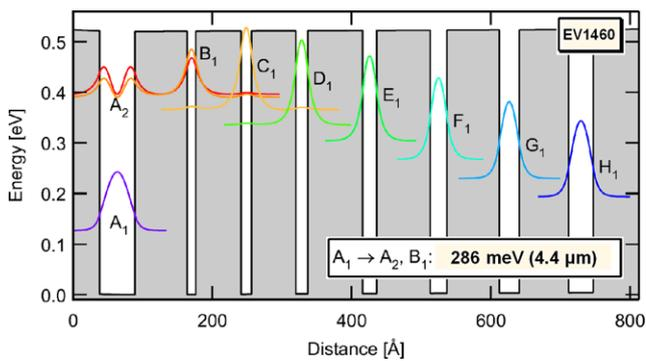
**Fig. 1** Schematic representation of one active region period of a typical QCD showing relevant wavefunctions and saw-tooth potential. The device presented in this article has a transition energy of 286 meV (4.4  $\mu\text{m}$ )
