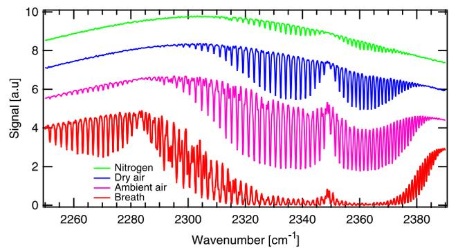
**Fig. 4** Comparison between different purge conditions. The *green*, *blue*, and *violet* curves correspond to CO<sub>2</sub>-concentrations of 10 ppm, 100 ppm, and 340 ppm, respectively. The *red* curve is for a much higher concentration, namely 5000 ppm. The resolution of these measurements was 0.25 cm<sup>-1</sup>
