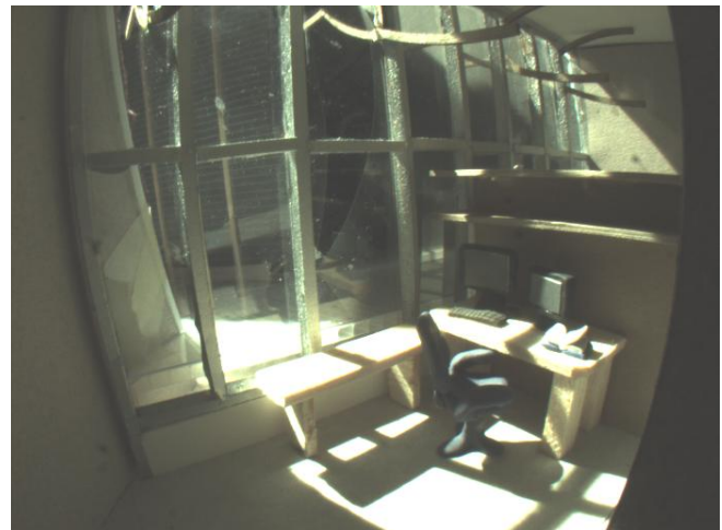
Fig 10: March 21 at 10 AM with a diffusing cloth covering the adjacent left exterior surface, cutting down on the reflections from the opposing structure.
