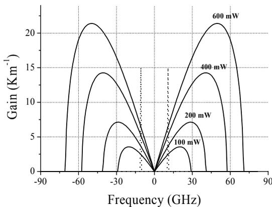
Fig. 1. Calculated gain spectra of MI for several power levels. The fibre parameters are  $\beta_2 = -21.9 \text{ ps}^2 \text{ km}^{-1}$  and  $\gamma = 1.78 \text{ W}^{-1} \text{ km}^{-1}$  at 1550 nm. Dotted lines indicate the position of modulated sidebands (at 10-11 GHz) for BOTDA sensing.
