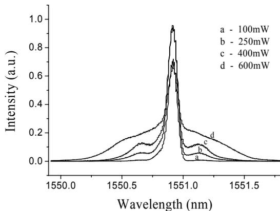
Fig. 4. Measured power spectra of spontaneous MI for a SMF in the anomalous dispersion region ( $\beta_2 < 0$ ). The input lightwave was a 20 ns pulse and the fibre was 11.8 km long.
