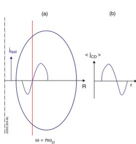
Figure 2. Current density profile driven by ICRF on the HFS through the Fisch mechanism (co-current propagating waves in this example)
