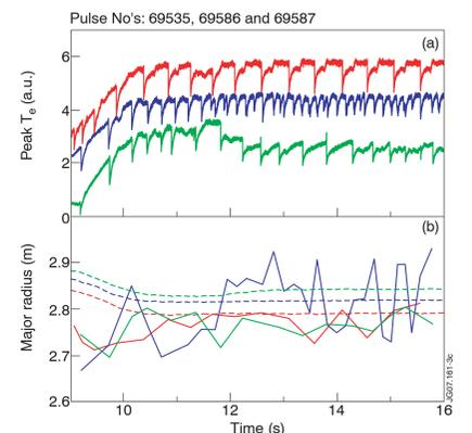
Figure 6. Comparison of three discharges differing by a variation of the toroidal magnetic field of less than 1%: the optimum for sawtooth stabilisation is the blue curve ( $B_T=2.83$  T); the green curve corresponds to  $B_T=2.85$  T and the red curve to  $B_T=2.81$  T. (In (b) the solid curves represent the inversion radius, the dashed curves the resonance radius.)
