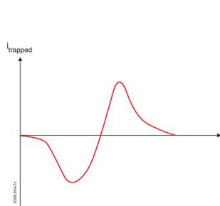
Figure 3. Current density profile driven by ICRF through trapped suprathermal ions owing to finite orbit width effects (direction is independent of antenna phasing)
