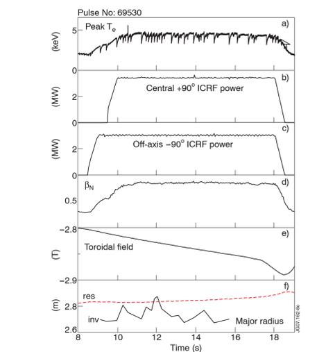
Figure 8.  $B_T$  sweep with no NBI heating. The optimum sawtooth stabilisation field in static conditions corresponds to the value reached here at 12 s, i.e. 2.83 T
