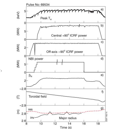
Figure 7.  $B_T$  sweep. The optimum sawtooth stabilisation field in static conditions corresponds to the value reached here at 13 s, i.e. 2.85 T
