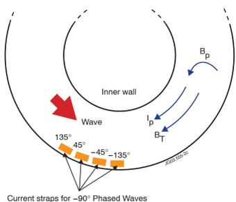
Figure 1. Schematic representation of one of the four ICRF antennae on JET. Each antenna has four current-carrying straps; the phasings of the currents in the straps determine the parallel wave-number spectrum, i.e., the wave directionality (counter-current propagation in the example shown, denoted as -90° phasing)
