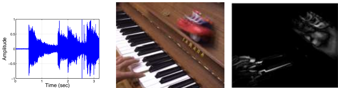
Fig. 5. Movie 1: Audio signal (left), sample raw frame (center) and corresponding dynamic pixels (right). Gray-levels on the right picture represent the absolute value of the difference image between two successive frames. Black pixels thus represent static regions.
