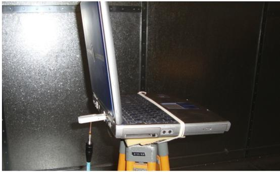
Fig. 2. Reverberation chamber setup for measuring the radiation efficiency of the antenna connected to a laptop computer.
