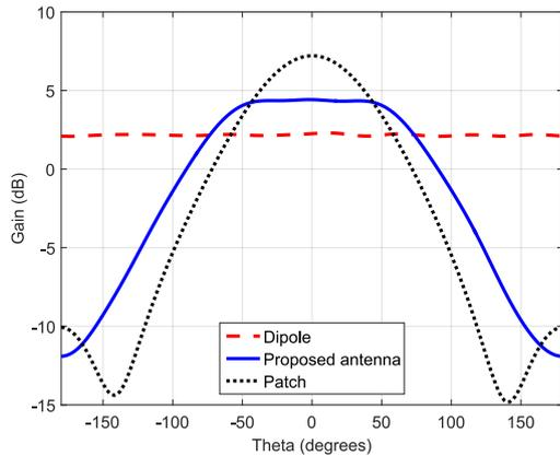
Fig. 7: Comparison of YZ pattern cut at 2.45GHz for the three antennas.
