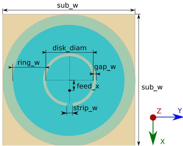
Fig. 2: Top view of antenna geometry.
