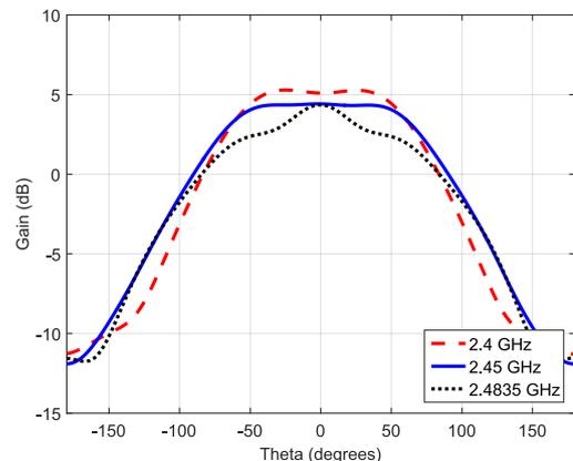
Fig. 5: Radiation pattern YZ cuts for the lowest, center, and highest frequency of the 2.4GHz ISM band.
