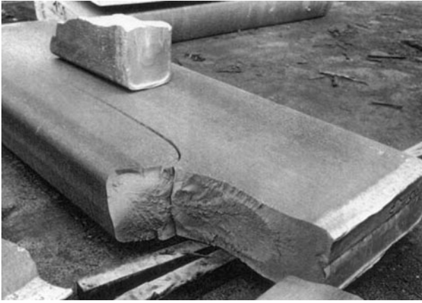
1 High strength aluminium alloy slab that cracked spontaneously during casting (cold cracking): 500 kg part that broke apart from ingot was projected several tens meters away; similar events can occur during sawing (photo courtesy Alcan)
