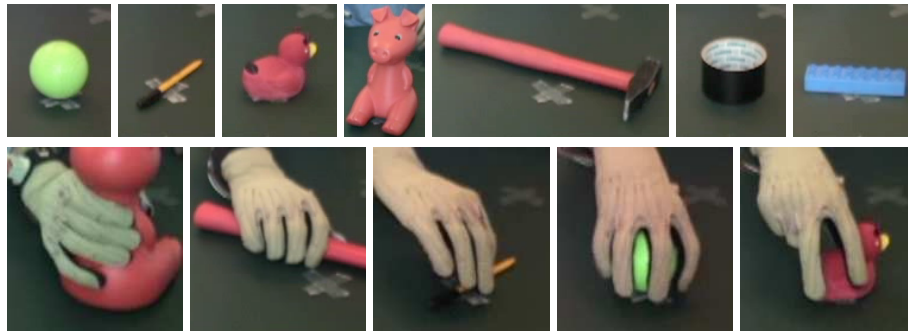
Fig. 3. Top row: the objects used in our experiments. Bottom, the grasp types we consider: (left to right) cylindrical power grasp, flat grasp, pinch grip, spherical and tripodal grip.
