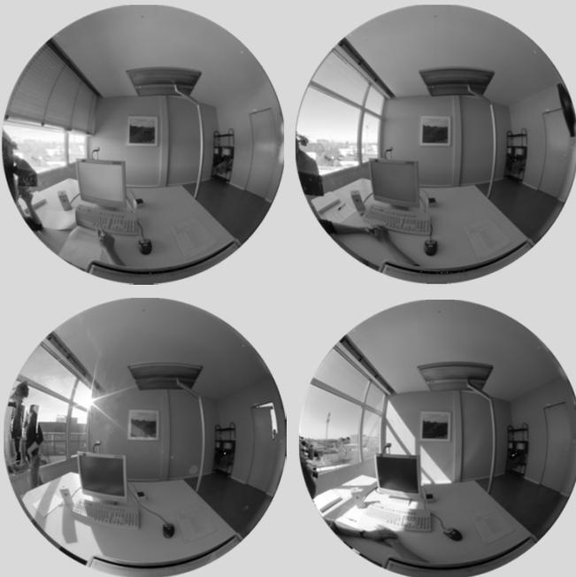
Daylit situation: Varying light conditions are created by setting four different facade configurations.
