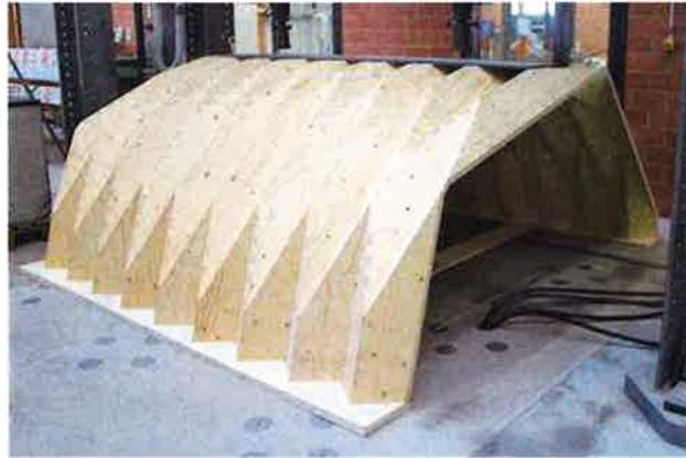
Fig. 7: Timber folded surface prototype
