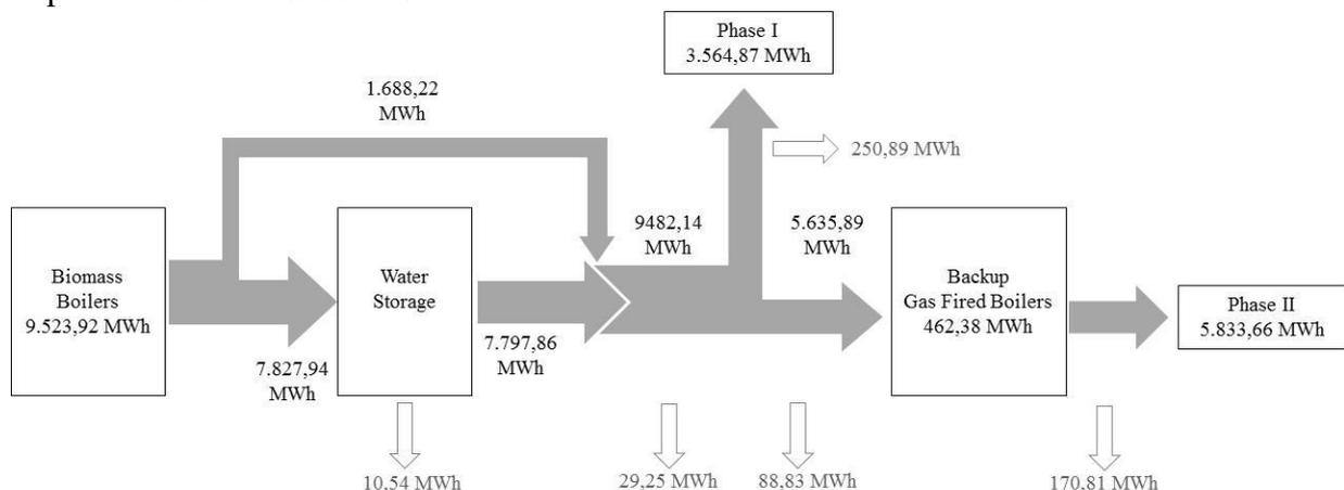
Figure 2: Biomass system simulation yearly energy balance.
