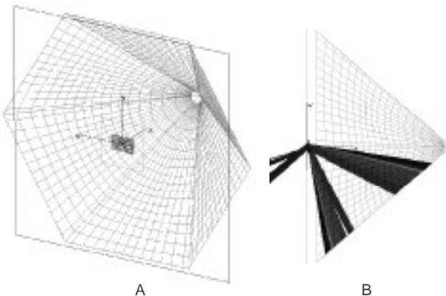
Fig. 1. (A) Simulation model, angular zones ( $\alpha_2$ ,  $\beta_2$ )=(5°, 5°). (B) Ray-tracing plots, incidence ( $\alpha_1$ ,  $\beta_1$ )=(40°, 90°).
