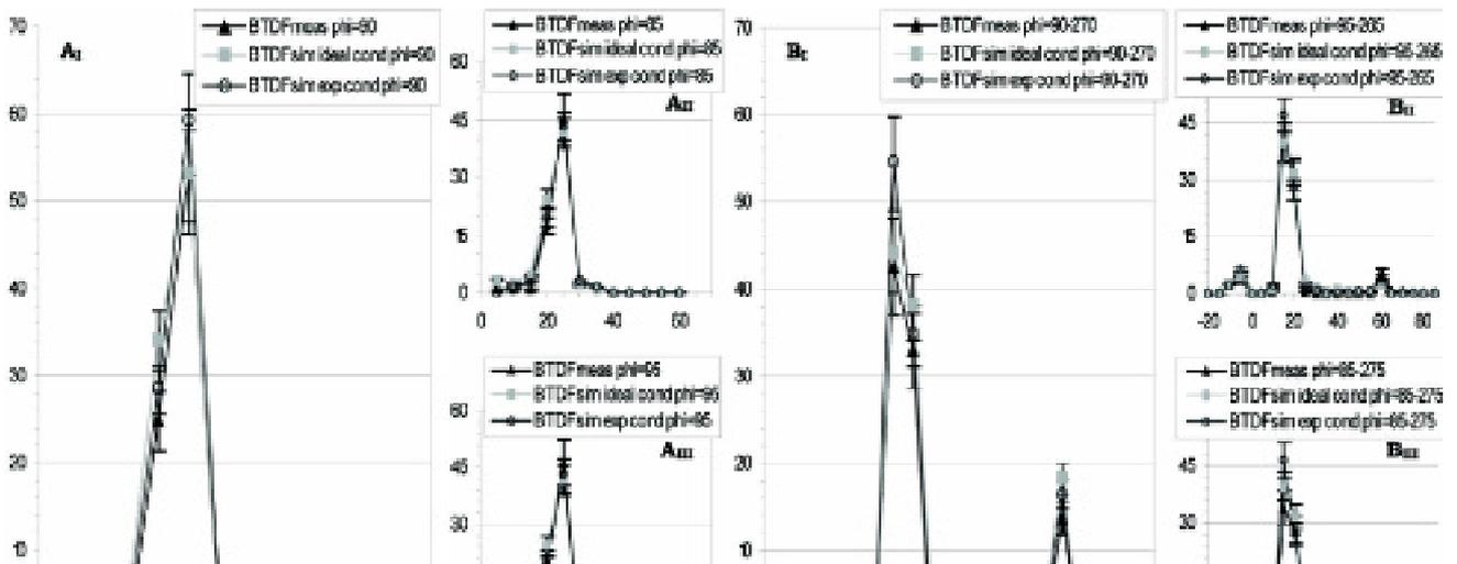
Fig. 3. BDF [ $\text{sr}^{-1}$ ] vs.  $\theta_2$  [ $^\circ$ ] along  $\theta_2$  planes: comparison of measurements (BTDFmeas) and calculations with experimental (BTDFsim exp) and ideal (BTDFsim ideal) conditions. (A) Asymmetric panel, gratings on incident side, incidence (0°, 0°). (B) Asymmetric panel, flat face on incident side, incidence (40°, 90°, 90°).
