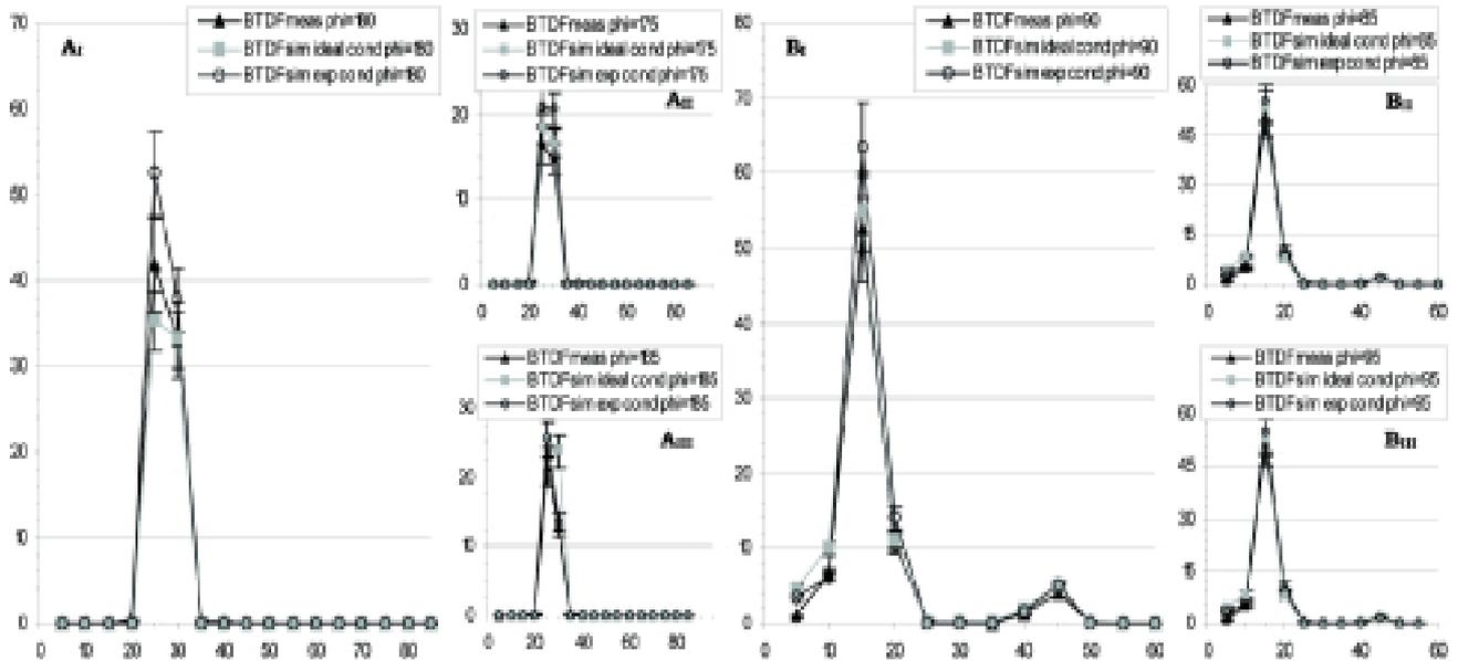
Fig. 2. BDF [ $\text{sr}^{-1}$ ] vs.  $\theta_2$  [ $^\circ$ ] along  $\theta_2$  planes: comparison of measurements (BTDFmeas) and calculations with experimental (BTDFsim exp) and ideal (BTDFsim ideal) conditions. (A) Symmetric panel, flat glass on incident side, incidence (40°, 45°). (B) Asymmetric panel, gratings on incident side, incidence (10°, 90°).
