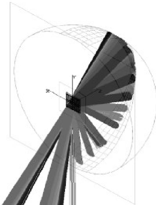
Fig. 4: Ideal simulation model hemispherical detector of adjusted radius. Asymmetric panel, Incidence ( $10^\circ, 90^\circ$ )
