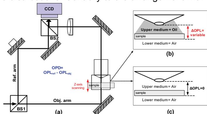
Fig. 1 (a) Simplified schematic of the HRIM. Close-up diagrams of the observation space (b) in oil and (c) in air.
