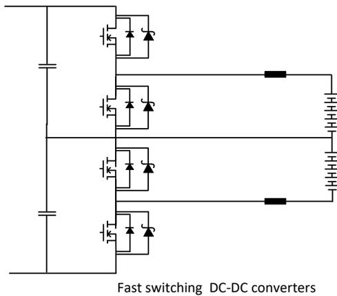
Fig. 5 Battery interface with SiC components
