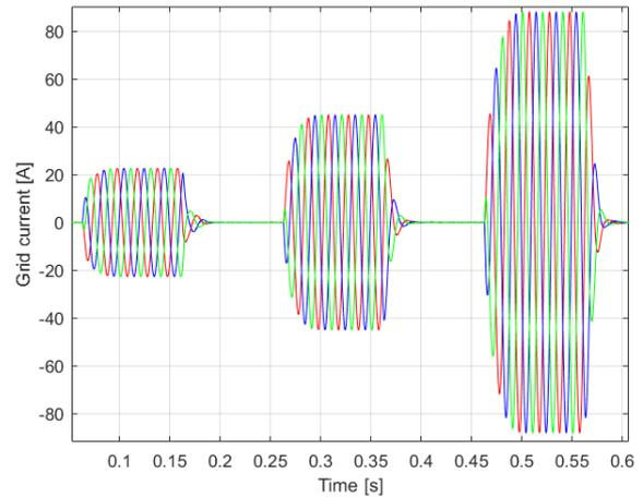
Fig. 9 AC-currents of the BBCU when charging the car at different power magnitudes
