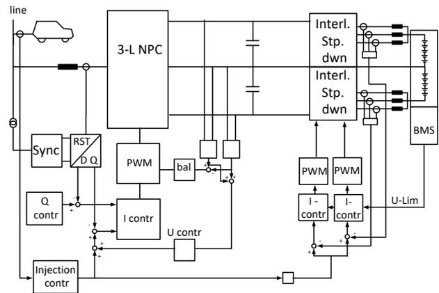
Fig. 6 Control diagram of the BBCU
