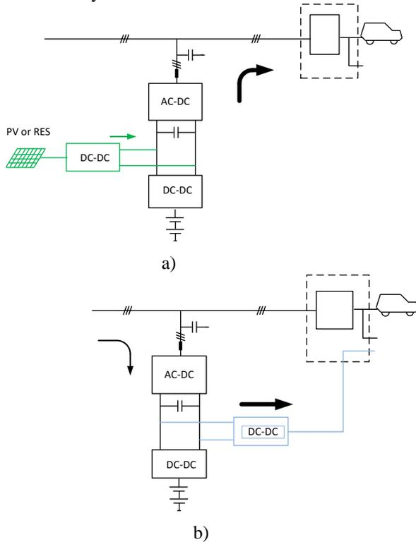
Fig. 2a) Integration with renewable sources, b) Extension for fast DC charging
