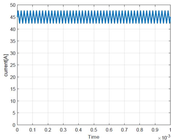
Fig. 11 Ripple of the current of the SiC based solution
