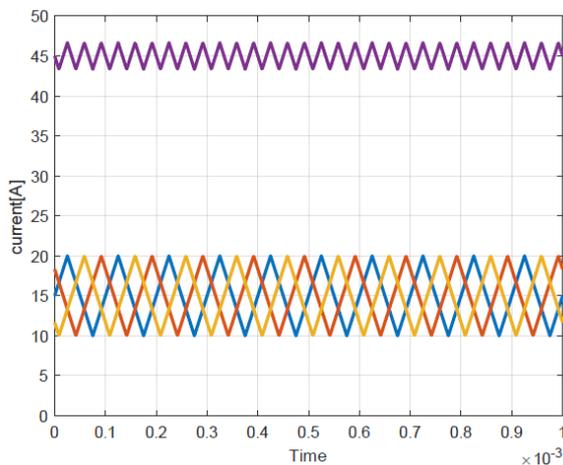
Fig. 12 Current ripples for battery and channels of the interleaved converter
