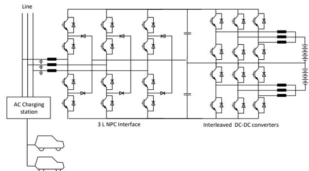
Fig. 4 The power circuits of the BBCU
