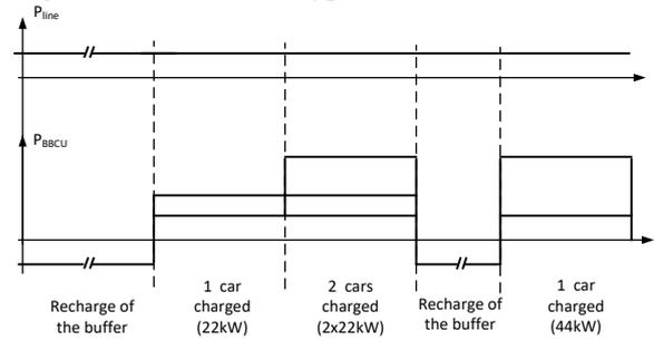
Fig. 3 Typical power cycles of the BBCU
