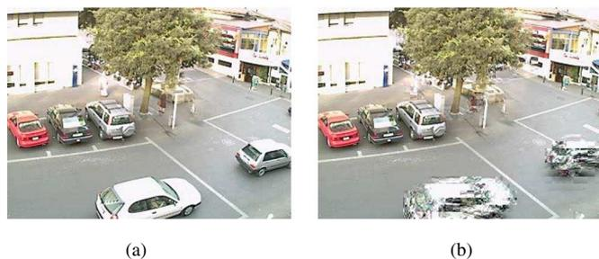
Fig. 11. Privacy protection scrambling in a real video surveillance setting: (a) original sequence and (b) with transform-domain scrambling.
