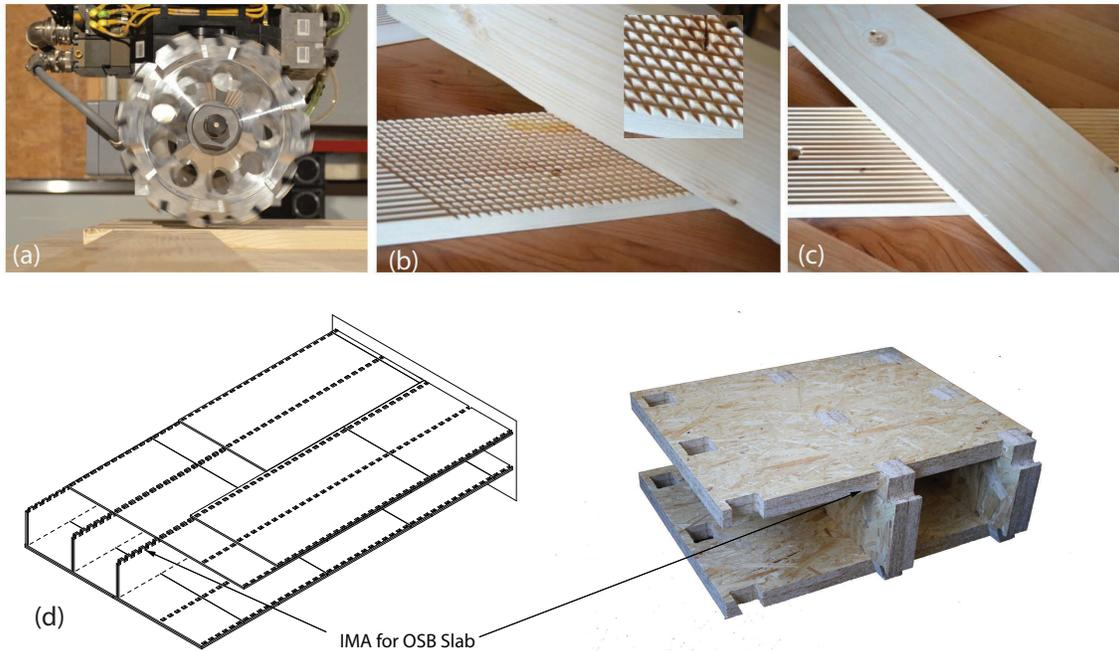
**Figure 1.** (a) Tool for mechanical preparation of wood interfaces on robot, (b) type of wood connection, (c) different angles possible, (d) IMA for slab made of OSB panels
