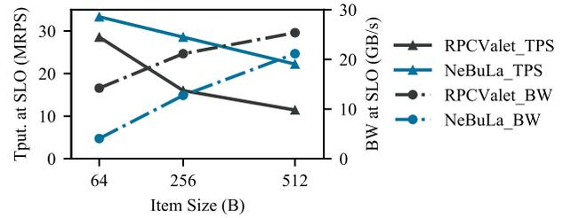
Fig. 7. Performance of RPCValet and NEBU<sub>A</sub> varying the MICA value size, using a 50/50 GET/SET query mix.
