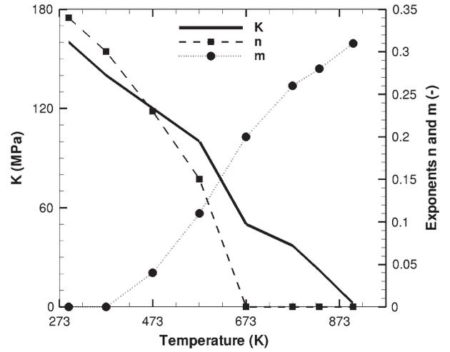
Fig. 4—Temperature variation of the consistency,  $K$ , and exponents,  $n$  and  $m$ , for the AA6063 alloy in the as-cast state.<sup>[24,25]</sup>
