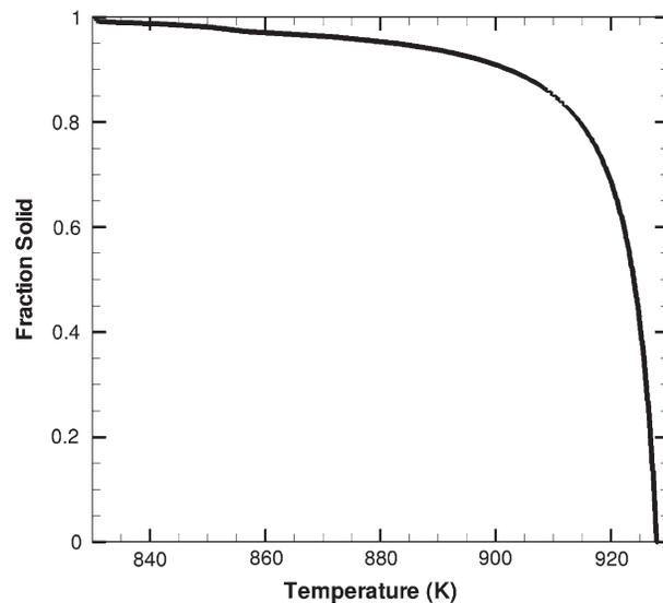
Fig. 2—Evolution in volume fraction solid with temperature for the AA6063 alloy.<sup>[23]</sup>
