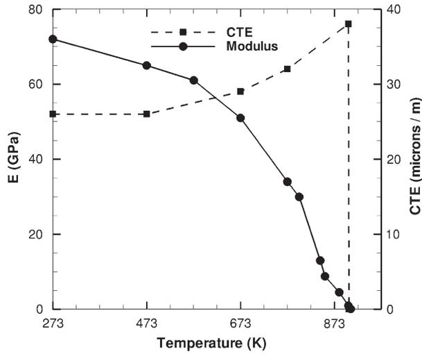
Fig. 3—Young's modulus (left scale) and CTE (right scale) vs temperature for the AA6063 alloy.<sup>[24,25]</sup>
