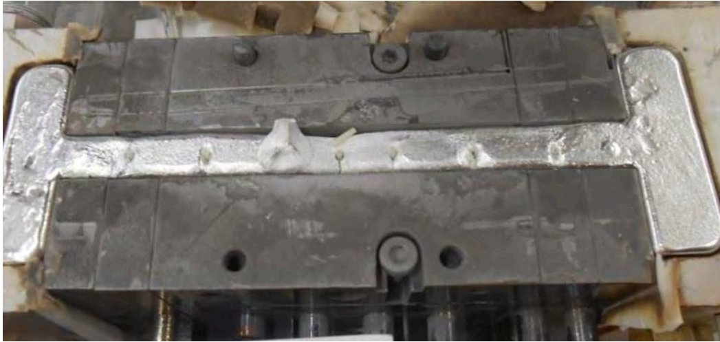
Figure 2: Sample DB3 showing a crack formed at the location of the thermocouple.
