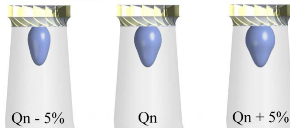
Fig.4 Variation of the vortex rope volume as function of the discharge
