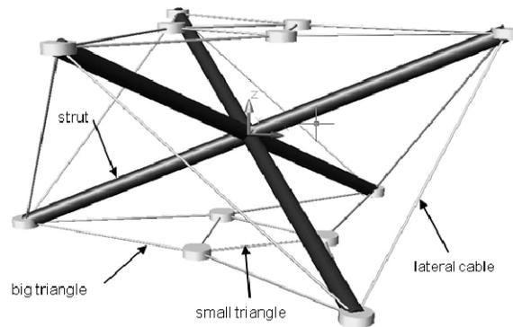
**Fig. 12.** Basic module of the tensegrity structure.
