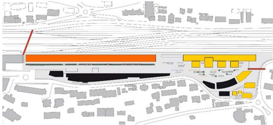
Figure 1. Site plan of Ecoparc at assessment. In black, buildings in operation. In yellow, buildings in execution phase. In orange, buildings in design phase. (Bauart document, 2005)
