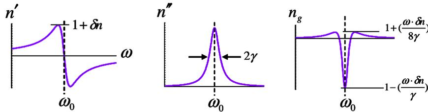
Fig. 1. Relation between the phase constant ( $n'$ ), the attenuation constant ( $n''$ ) and the group index ( $n_g$ ) around the absorption peak centered at  $\omega_0$ .
