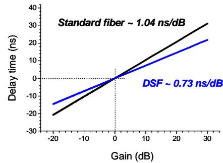
Fig. 2-(b) Delay time as a function of Brillouin gain..
