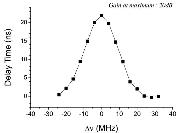
Fig. 6. Delay time of the probe pulse as a function of the modulation frequency deviation ( $\Delta\nu$ ) from  $\nu_B$ . The pump and the probe powers were fixed.
