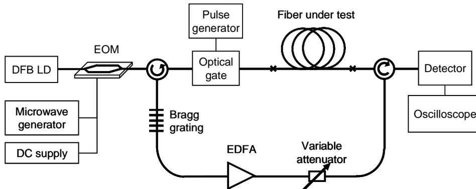
Fig. 3. Configuration to measure variable pulse delay from SBS in an optical fiber
