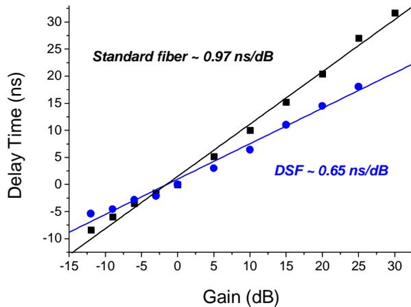
Fig. 5. Delay time of the pulse as a function of the Brillouin gain. In a gain situation the pulse is delayed while it is accelerated in a loss configuration.
