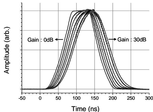
Fig. 4. Traces of the probe pulses for different Brillouin gains (standard fiber), showing a clear delay due to the modified group velocity.
