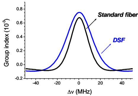
Fig. 2-(a) Group index variation according to frequency deviation from Brillouin frequency. The gain is 20dB when  $\Delta\nu = 0$
