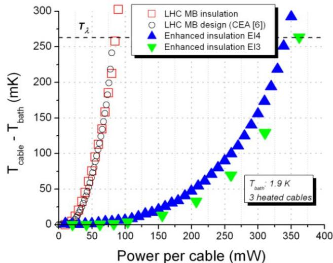
Figure 3 Cable temperature increase vs. power dissipated in the central conductor, in He bath at 1.9 K
