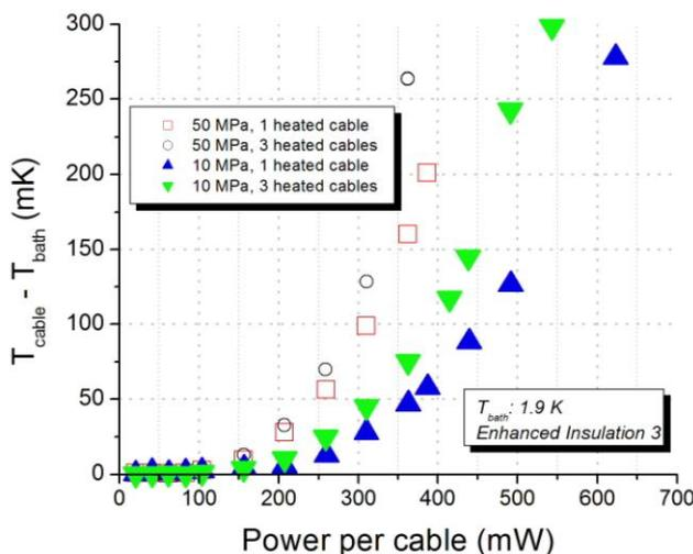
Figure 5 Cable temperature increase vs. power dissipated in the central conductor for EI3, in He bath at 1.9 K.
