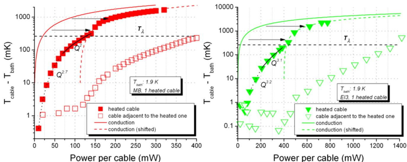
Figure 4 Cable temperature increase vs. power dissipated in the central conductor, in He bath at 1.9 K. MB insulation on the left, EI3 on the right. The conduction curves are shown, as well as the power laws fitting the measurements below 300 mK
