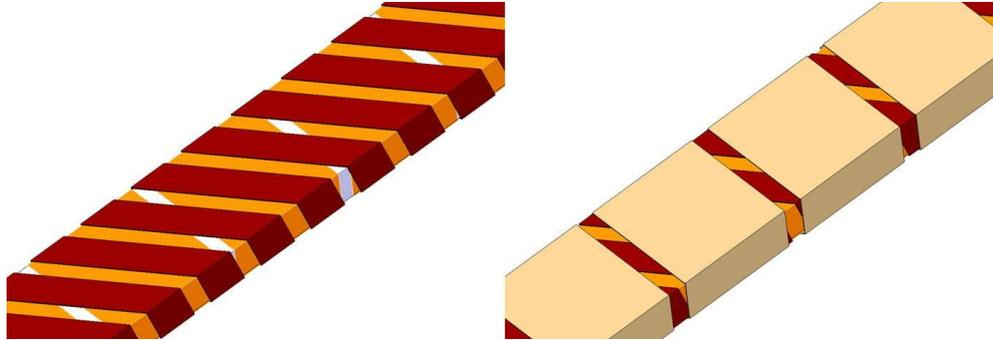
Figure 1 Scheme of the Enhanced Insulation: the 1<sup>st</sup> and 2<sup>nd</sup> tapes are shown on the left, whereas all the tapes are shown on the right.
