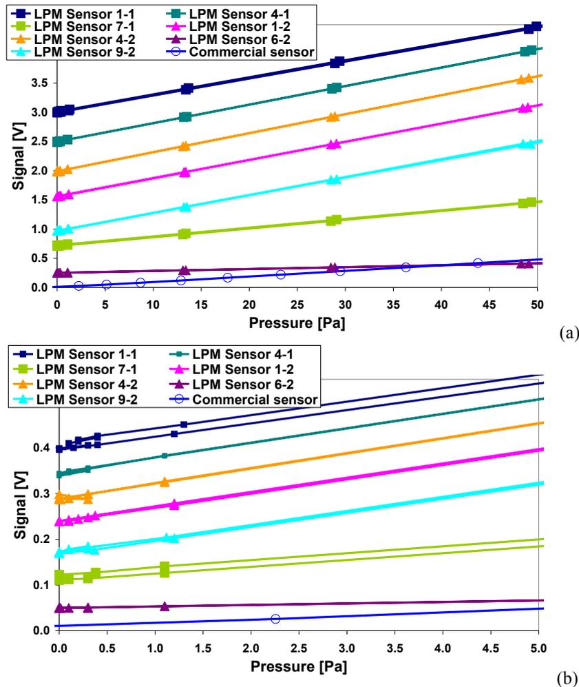
Fig. 5: Signal of different sensors assembled with the Venturi tube as a function of the pressure (a), with zoom for low flows in (b). Output signals shifted for better readability.
