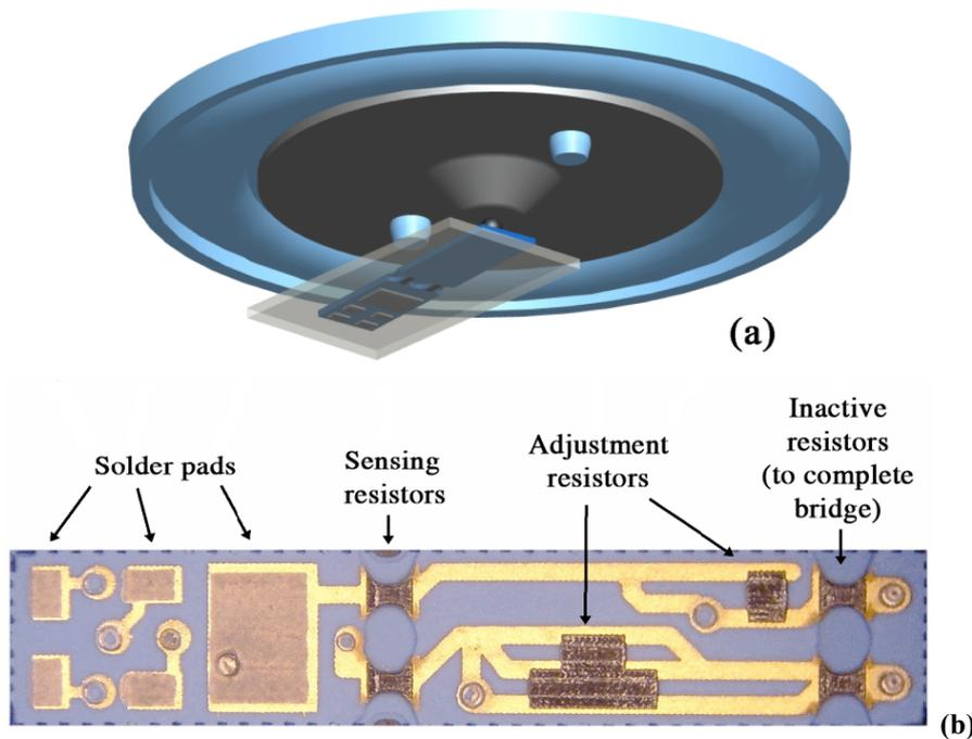
Fig. 3. (a) elastomer membrane with reinforcing central structure mounted on LTCC cantilever sensor; (b) LTCC cantilever - bottom side.
