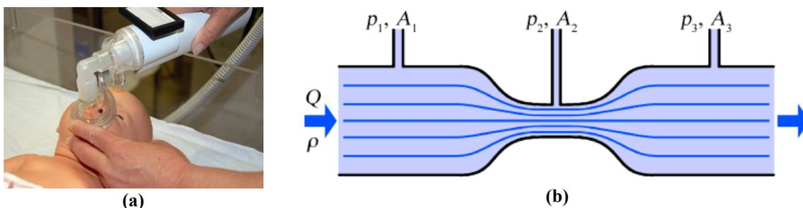
Fig.1. (a) neonatal respiratory assistance (source: [www.kmedical.co.nz](http://www.kmedical.co.nz)); (b) Working principle of Venturi tube used to convert flow into pressure.
