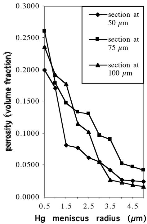
Fig. 10: Cumulative pore size distribution curves determined from using the numerical Mercury Porosimetry Technique on the 2D image.
