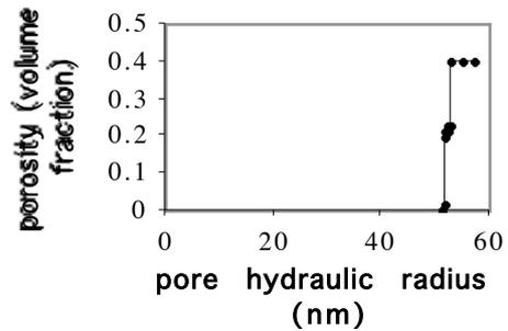
Fig. 8: Cumulative pore-size curve of closed-packed silica spheres pore structure.
