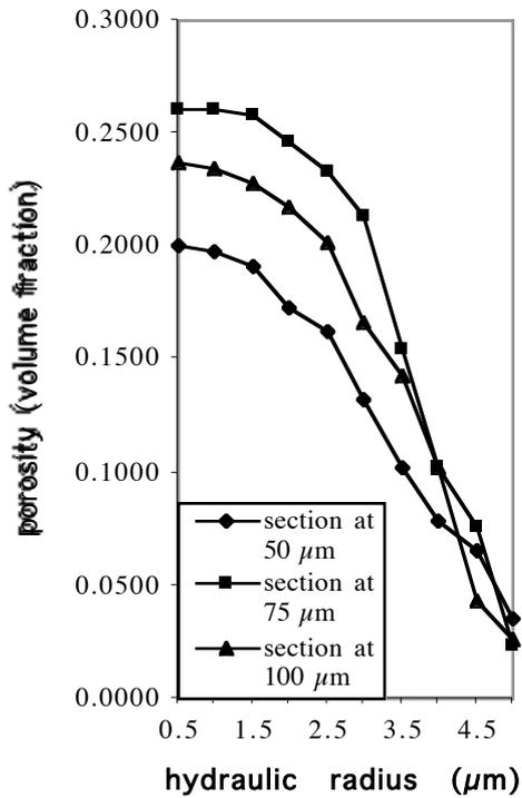
Fig. 12: Cumulative pore size curves obtained for 3 sections at 50, 75 and 100 micrometers distance from the boundary of computational volume, using the MTPVS.
