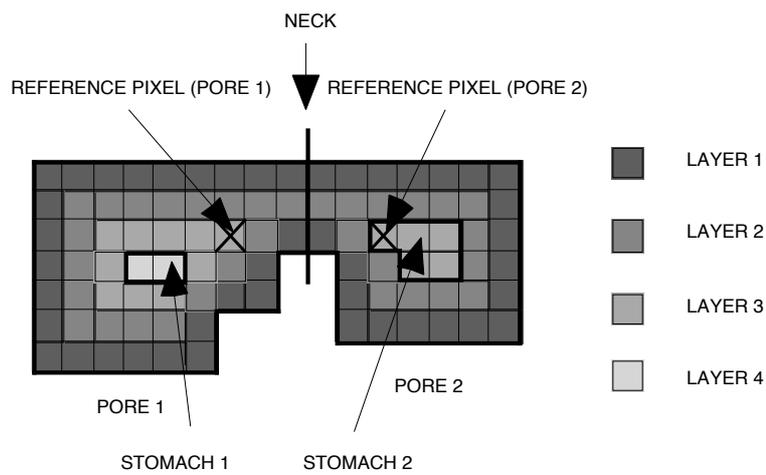
Fig. 2: Partitioning of the pore space into pore 1 and pore 2.
