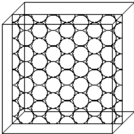
Fig. 7: Schematic representation of computational volume,  $2170 \times 2170 \times 2170 \text{ nm}^3$  with periodic boundary conditions, consisting of pores and spherical particles. A 2D slice is cut through the middle of spheres
