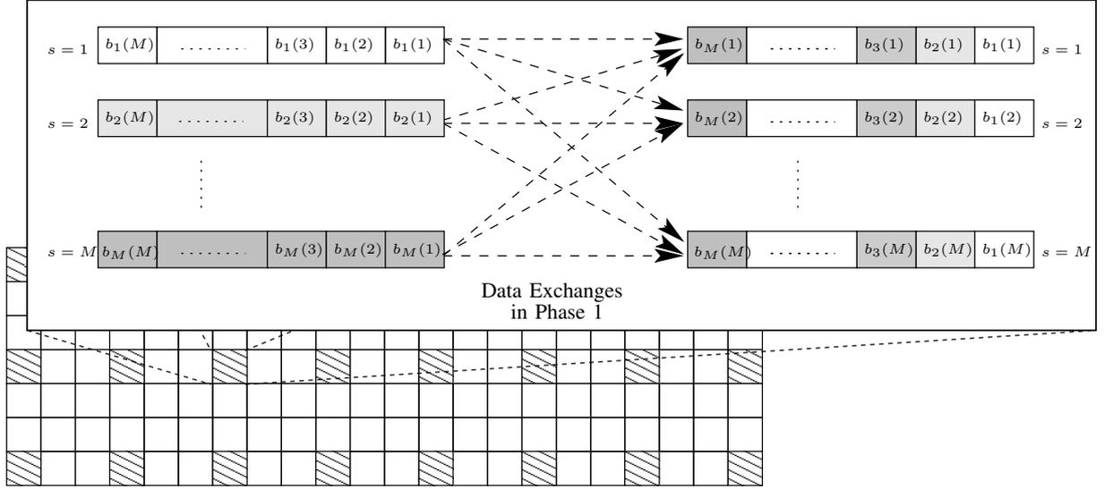
Fig. 4. Buffers of the nodes in a cluster are illustrated before and after the data exchanges in Phase 1. The data stream of the source nodes are distributed to the  $M$  nodes in the network as depicted.  $b_s(j)$  denotes the  $j$ 'th sub-block of the source node  $s$ . Note the 9-TDMA scheme that is employed over the network in this phase.
