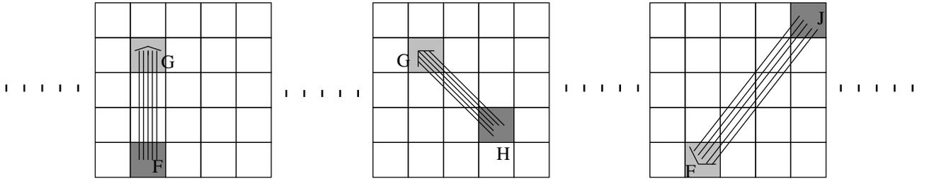
Fig. 2. Successive MIMO transmissions are performed between clusters. The first figure depicts MIMO transmission from cluster  $F$  to  $G$ , where bits originally belonging to  $s_1$  are simultaneously transmitted by all nodes in  $F$  to all nodes in  $G$ . The second MIMO transmission is from  $H$  to  $G$ , while now bits of source node  $s_2$  are transmitted by nodes in  $H$  to nodes in  $G$ . The third picture illustrates MIMO transmission from cluster  $J$  to  $F$ .
