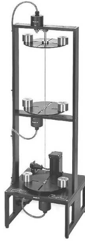
Figure 6. Torsional setup, ECP Model 205
