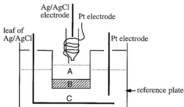
**Fig. 1.** Schematic representation of the principle of the 96-well microfilter plates system. A, Aqueous phase 250  $\mu\text{L}$  at fixed pH containing the drug; B, polyvinylidene difluoride membrane with nitrophenyloctyl ether solvent; C, Aqueous reference phase
