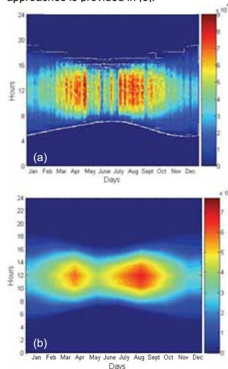
Figure 2. Temporal Maps for a North-facing façade in Sydney displaying outside vertical illuminance in lux, based on (a) five minutes intervals using DAYSIM and (b) a reduced set of 56 data points for Lightsolve
