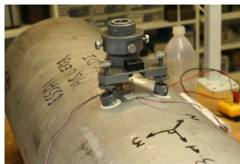
2 Measurement of surface residual stresses using hole drilling method
